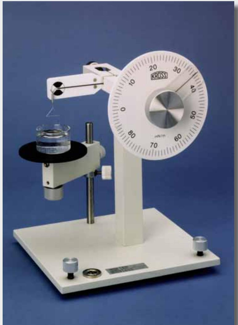
KRÜSS tensiometer with all advantages for a rapid and simple determination of the surface tension of liquids
